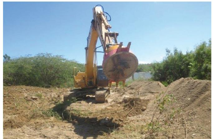
*Magnetic attachment on excavator removing bombs from the roadbed. In areas where it is too dangerous or costly to remove munitions by traditional methods, remotely operated equipment has significantly reduced explosive hazards to workers and cut costs by more than half.*
