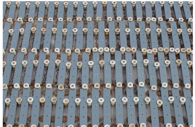
*Outdoor exposure test coupons for seven hexavalent chromium-free surface paint systems are set up for long exposure tests. Tests are conducted under high humidity, rainfall, and salt conditions in Daytona, Florida.*
